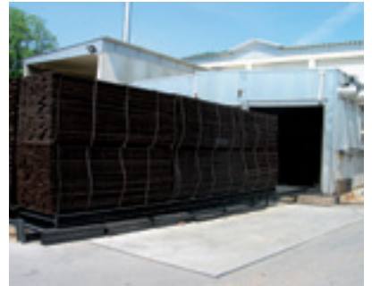
The woods for Redecker's Thermowood products are heated for a day in large kilns.
