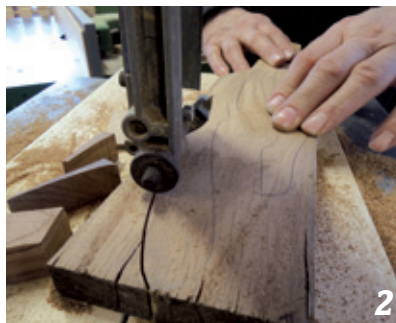
2 Each shape is cut individually from the beam, with conscious consideration of the characteristics of the piece.
